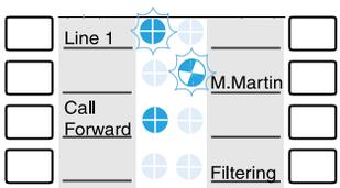
**Icons associated with the programmable keys.** These allow you to view the status of the line or the programmed function:
